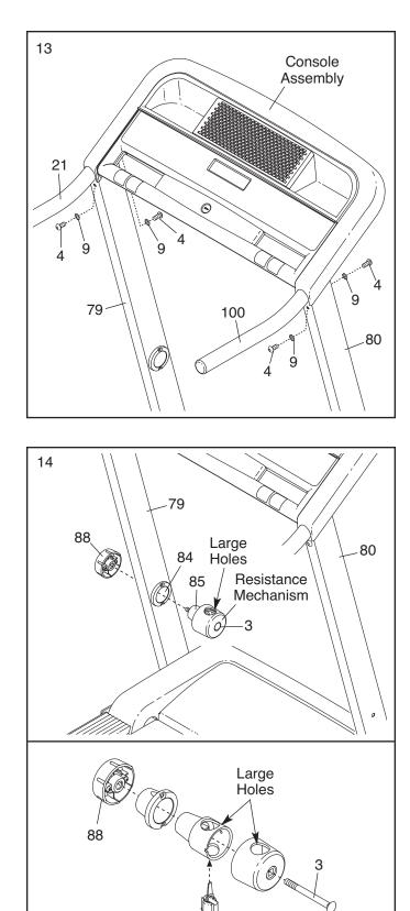
14. Remove the Resistance Knob (88) from a resistance mechanism. Make sure that the 3/8" x 4 3/4" Bolt (3) stays inside the resistance mechanism and that the resistance mechanism does not come apart. Note: See the lower drawing to reassemble the resistance mechanism if necessary.
